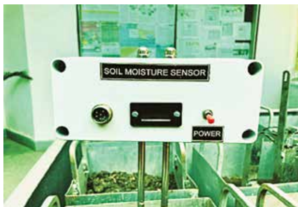
Capacitance based soil moisture sensor FDR+ Capacitance based soil moisture sensor
